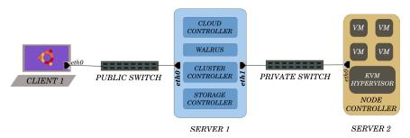
Figure 2.1: UEC basic setup with three machines
